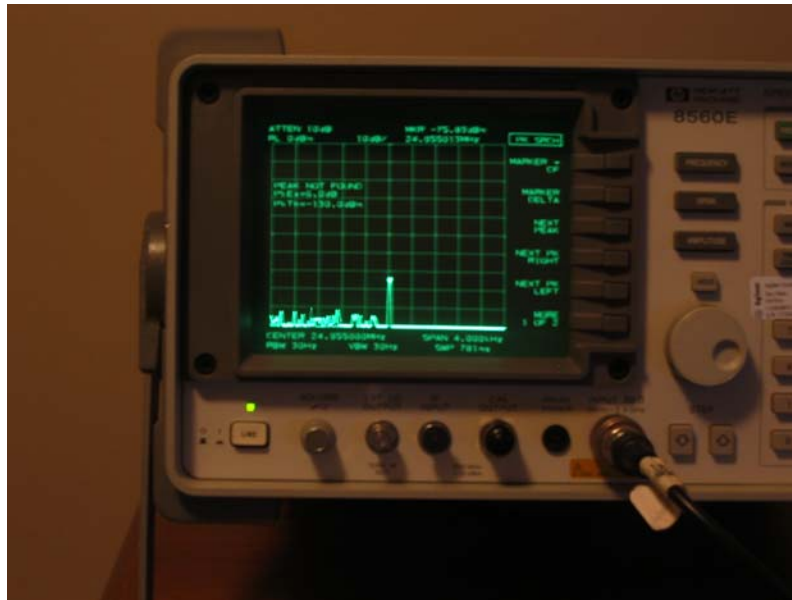
Picture 29: LSB Carrier Suppression after Mod
